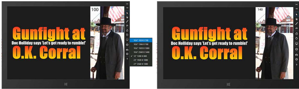
Figure 28 – You can test the auto image resolution in the Simulator. The project is displayed on a simulated 1280x800 device on the left and a simulated 1920x1080 device on the right. The left device uses the 100 scale version and the right uses the 140 scale version of the graphic. TIP: To test, you must change the resolution of the simulator, end the project, and re-launch it to display the correct scale. In this example, the 100 and 140 numbers are part of the graphic.
