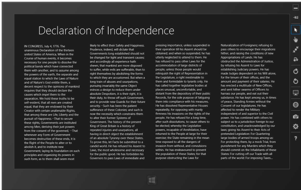
Figure 21 – RichTextBlockOverflow controls are utilized to have text flow from one control to the other.
