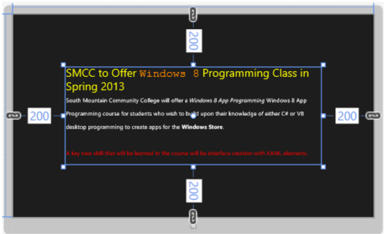
Figure 19 – Formatting can be set within individual <Paragraph> tags of a RichTextBlock . Inline tags such as <Bold> and <Italic> may also be applied.
